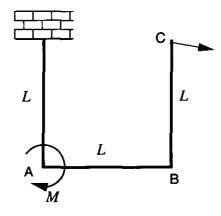
a. Express the displacement vector at point C in terms of M, L and the bending stiffness E1.
