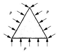
For a finite element analysis, the body is meshed with triangular elements, so that each of the three boundary edges contains N nodes. These nodes are connected along each edge by N-1 elements, inside of which the displacements are interpolated by linear shape functions  $N^I(s)$ , where s is a coordinate along an edge from one corner of the triangle to the other.
